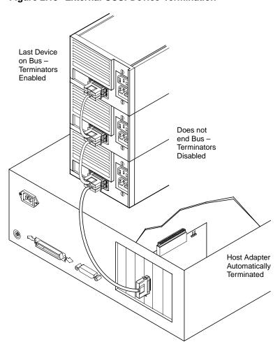
Figure 2.13 External SCSI Device Termination
